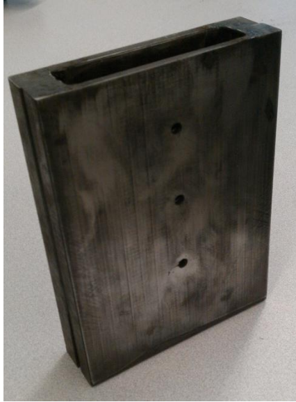
Figure 3.12: Photograph of completed and assembled mold.
