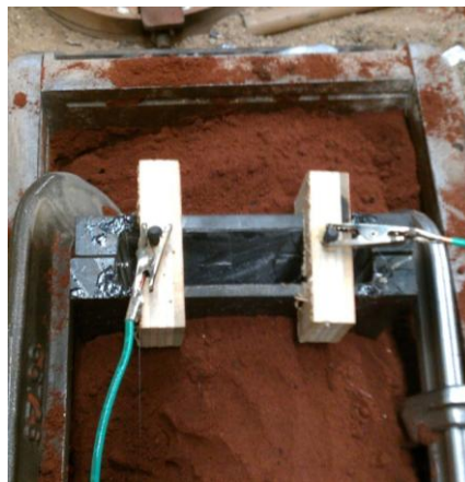
Figure 3.7: Photograph of the electrode setup at the mold prior to pouring.
