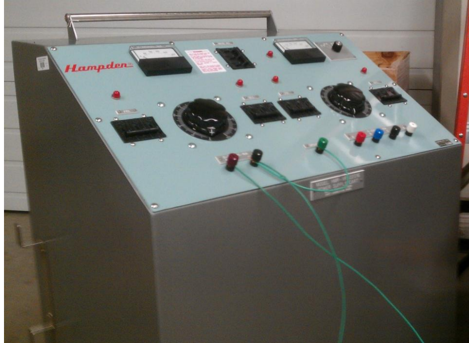
Figure 3.8: Photograph of the power supply used to apply the electric current.
