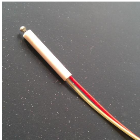
Figure 3.4: K type thermocouple with ceramic sleeve used for temperature measurement during solidification.
