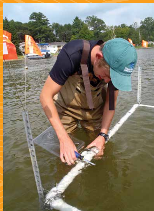
Graduate student James Smit setting up a bioassay experiment in Silver Lake, MI, to determine algal responses to additions of nitrogen and phosphorus.
