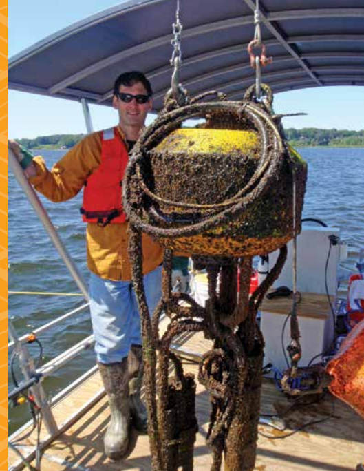
AWRI research assistant Scott Kendall brings up the submerged Muskegon Lake Buoy Observatory for a mid-summer sensor check and mussel removal.
