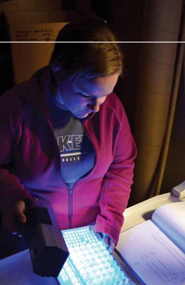
Graduate student Sarah Stamann conducts E. coli measurements of Flat River samples using the Colilert method.
